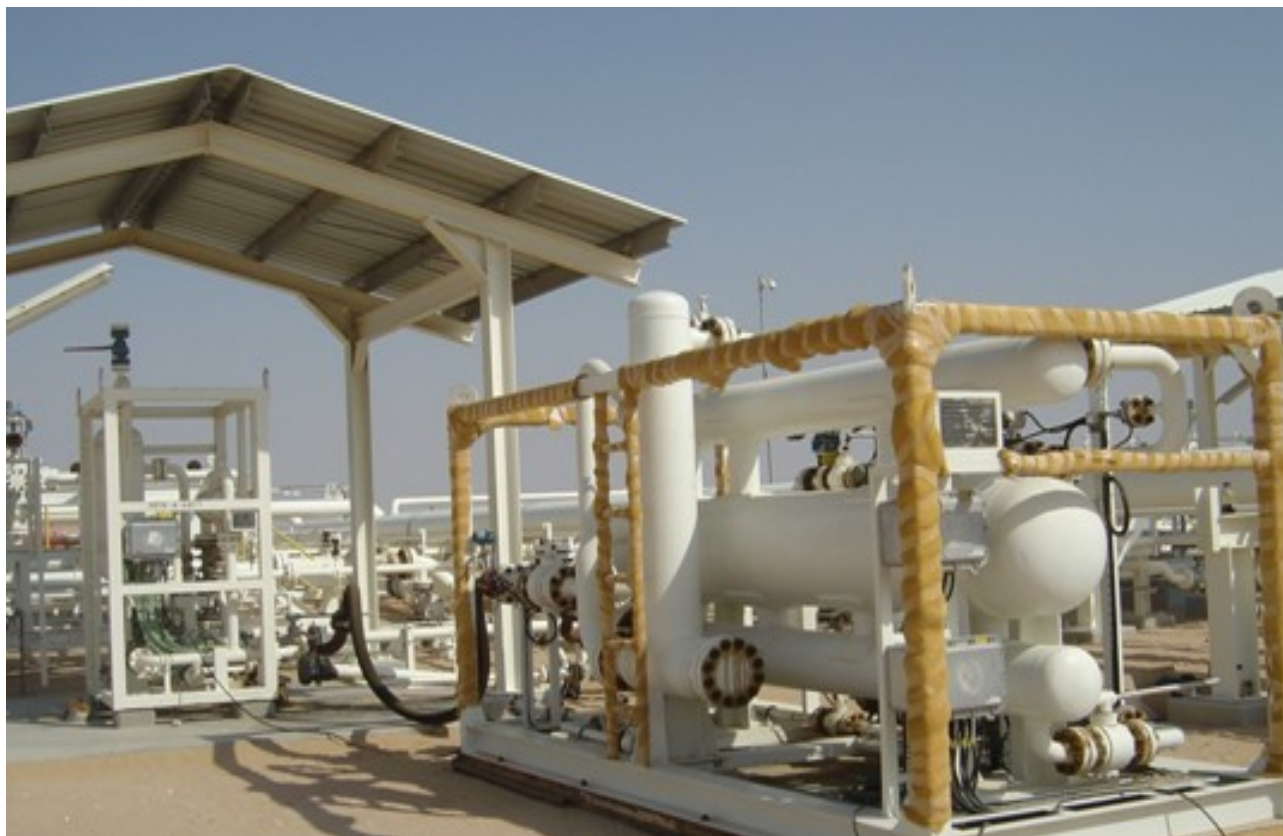
Fig. 4 - HPT & MPFM Setup for Validation Test
